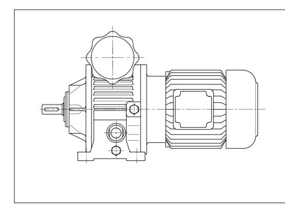
G\_\_\_ motion DISCO variable speed drive
